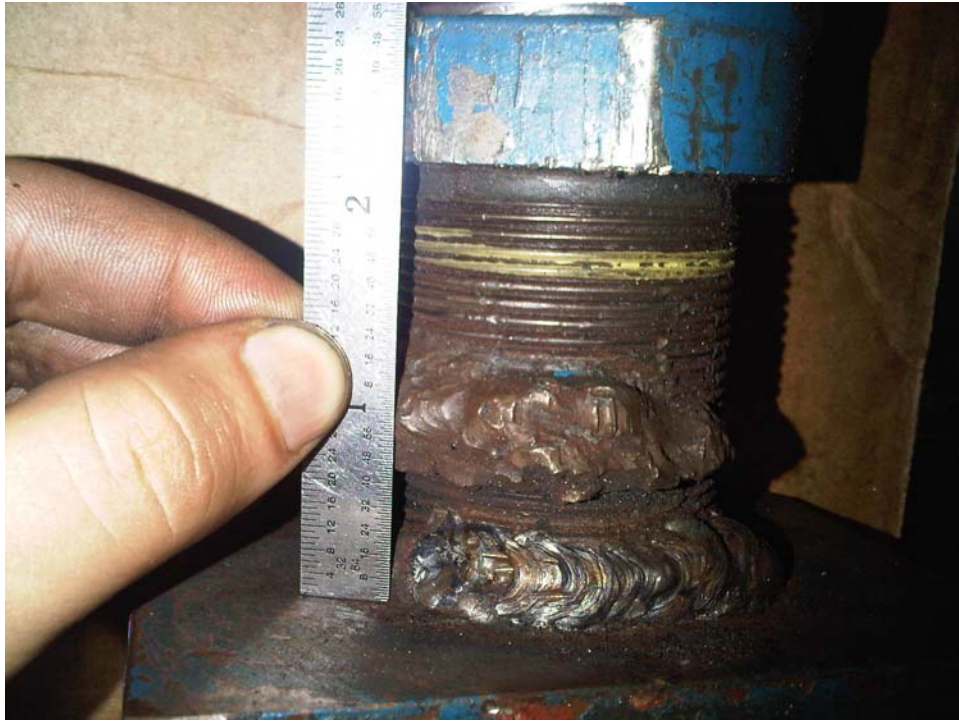
Figure 2.2 – Image of Failed Threads Showing ¼” Engagement
